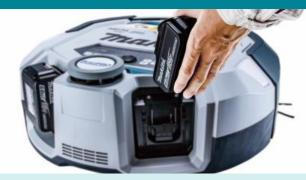
Parallel 18V batteries provide extended runtime for large cleaning areas
