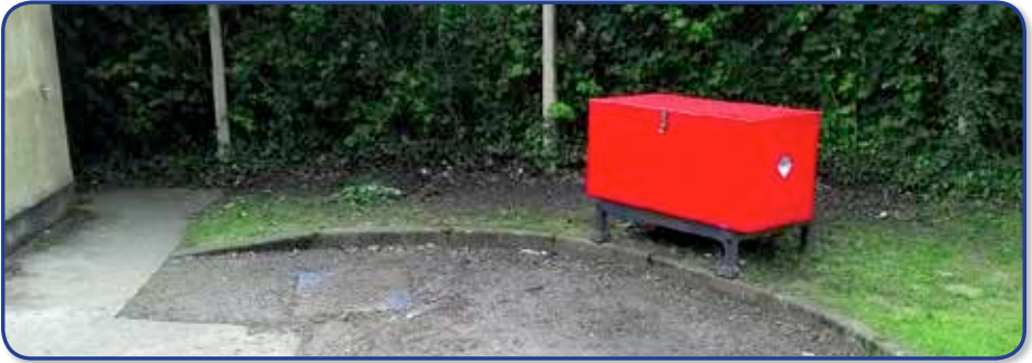
An example of a waste battery storage bin well away from buildings.
